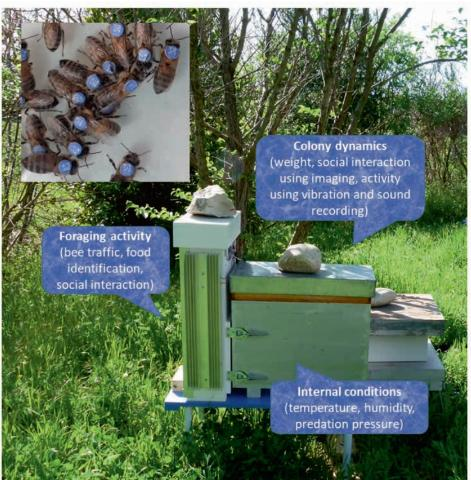
◀ A digitally connected beehive monitoring system providing information on the colony health and, more broadly, on the quality of the foraging environment.
