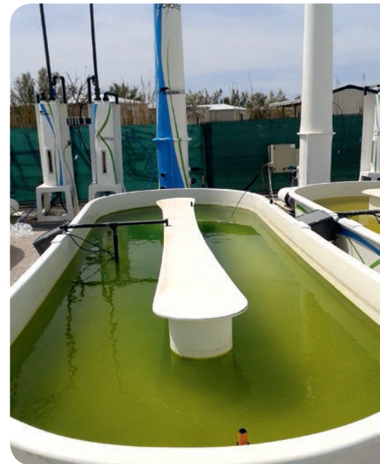
▲ High rate algal pond for experiments on industrial fume remediation (IFREMER platform, Palavas, France). © Éric Fouilland
