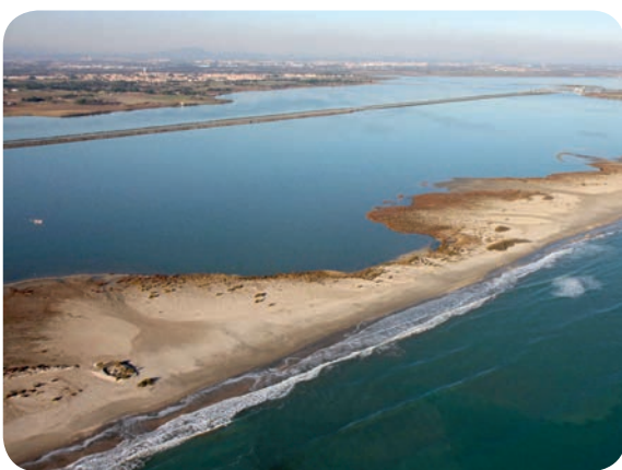
◀ Fig. 2. The Maguelone coastline, showing storm deposits on the lagoon during stormy periods, which are causing gradual shoreline displacement towards the piedmont, with a constant sand volume on the coast. © DREAL
