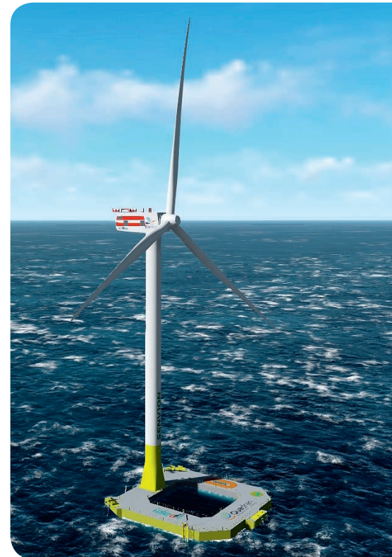
▲ Representation (synthetic image) of a floating wind turbine installed on a semi-submersible platform. © Quadran Énergies Marines
