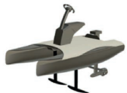
▲ View of an Overboat – the first electric boat with regulated foils for the general public. It is the size of a jet ski while being perfectly silent, stable and very energy-efficient. © NEOCEAN
