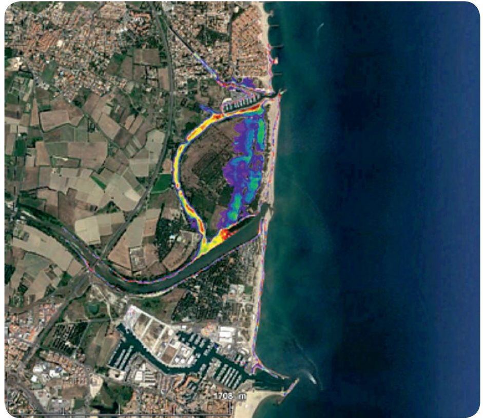
▲ Modelling flooding due to Têt River overflow (Pyrénées-Orientales region) and marine submersion. The colours highlight water-covered areas. Here the flooded areas correspond mainly to the former Têt riverbed and no-build zones between the former and current riverbeds. © P. Marsaleix/Aerology Laboratory
