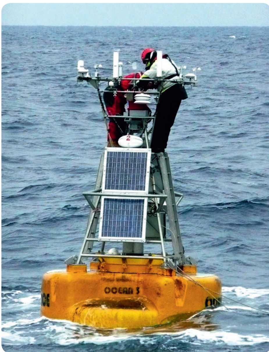
▲ Installation of new sensors in the framework of the HyMeX programme on the Météo-France fixed buoy in the Gulf of Lion. © CNRM
