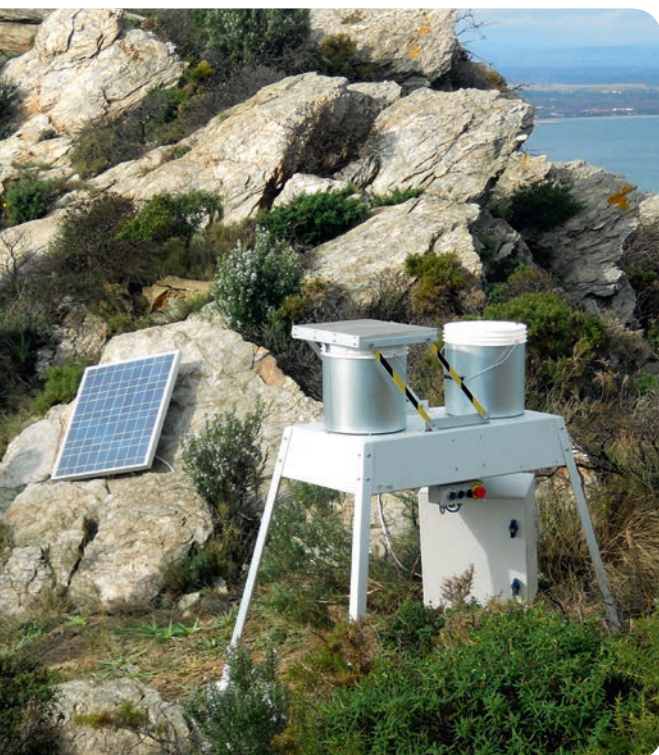
▲ Atmospheric deposition collecting system at Cap Béar, France. © D. Aubert
