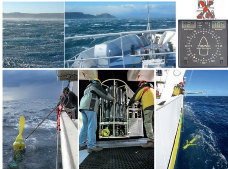
▲ The DeWEX initiative during the winter of 2012-2013 (upper band) combined autonomous platform approaches with drifting buoys, underwater gliders (right and left photos in the lower band) and sampling surveys aboard oceanographic vessels (central photo of the lower band, launch of a rosette sampler with 12 Niskin bottles). © Conan Pascal
